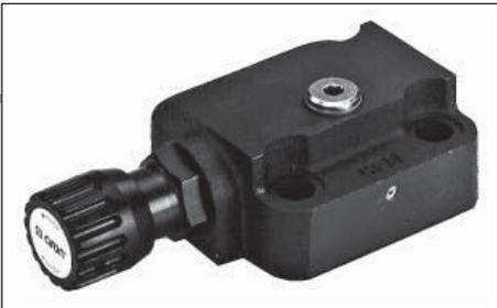
Aron maximum pressure cartridge valves allow control of hydraulic circuit pressures up to 400 bar and 350 l/min maximum flow rate (NG25). Besides the normal manual pressure regulation mode, function like electrical command for discharge to drain, remote control, proportional pressure control or electrically selected dual pressure levels are also available.
