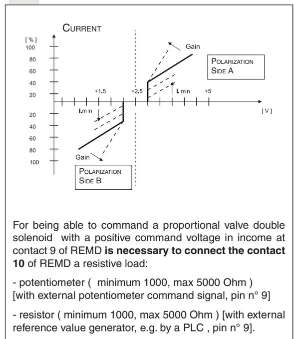
For being able to command a proportional valve double solenoid with a positive command voltage in income at contact 9 of REMD **is necessary to connect the contact 10** of REMD a resistive load:
