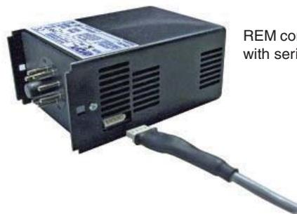
REM connecting at computer with serial cable.
