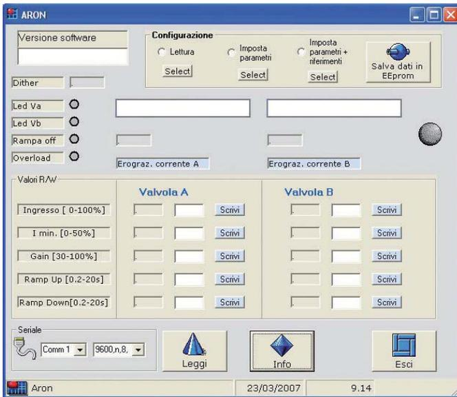
AronDG program for the digital adjustment of the parameters of the REMS and REMD boards.
