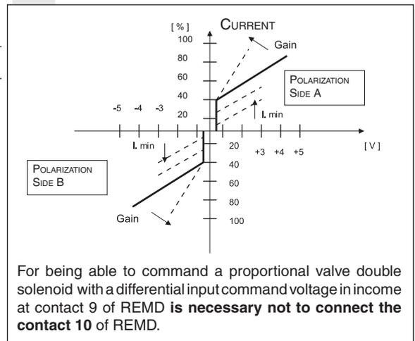
For being able to command a proportional valve double solenoid with a differential input command voltage in income at contact 9 of REMD **is necessary not to connect the contact 10** of REMD.
